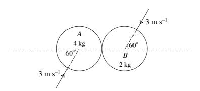
Two uniform smooth spheres A and B, of equal radius, have masses 4 kg and 2 kg respectively. They are moving on a horizontal surface when they collide. Immediately before the collision both spheres have speed 3 m s<sup>-1</sup>. The spheres are moving in opposite directions, each at  $60^{\circ}$  to the line of centres (see diagram). After the collision A moves in a direction perpendicular to the line of centres.
