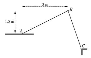
Two uniform rods, AB and BC, are freely jointed to each other at B, and C is freely jointed to a fixed point. The rods are in equilibrium in a vertical plane with A resting on a rough horizontal surface. This surface is 1.5 m below the level of B and the horizontal distance between A and B is 3 m (see diagram). The weight of AB is 80 N and the frictional force acting on AB at A is 14 N.
